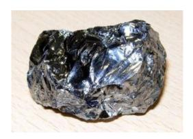
Silicon (Atomic number 14) is an important element in electronics
